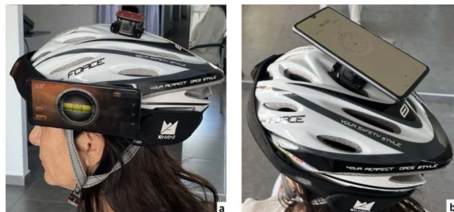
Figure 1. Details of placement of both devices on a helmet fastened securely to the participants' heads. Placement of mobile phone to the side (a), and on top (b) of the helmet.
