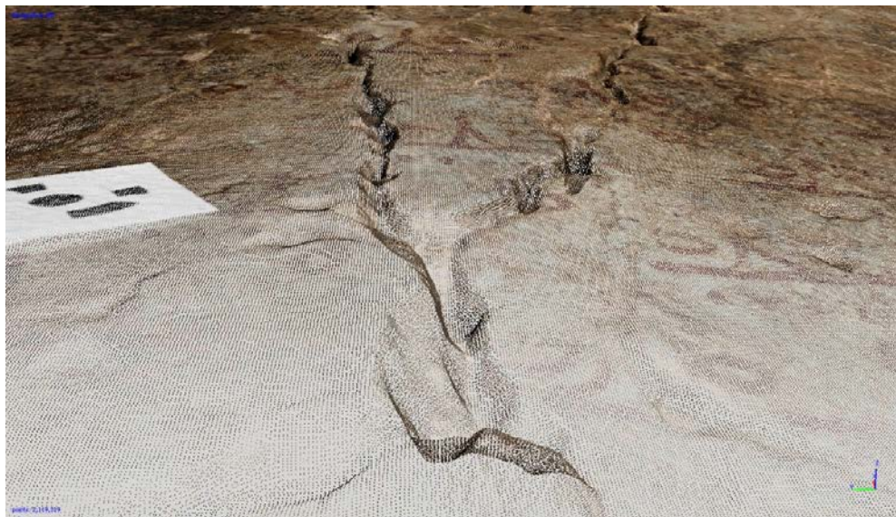
Figure 9. Detailed view of the dense point cloud corresponding to the area depicted in Figure 8d–f. The point cloud consists of points in a three-dimensional space, each carrying color information derived from the source images, providing a high-fidelity representation of the mural's geometry and chromatic characteristics.
