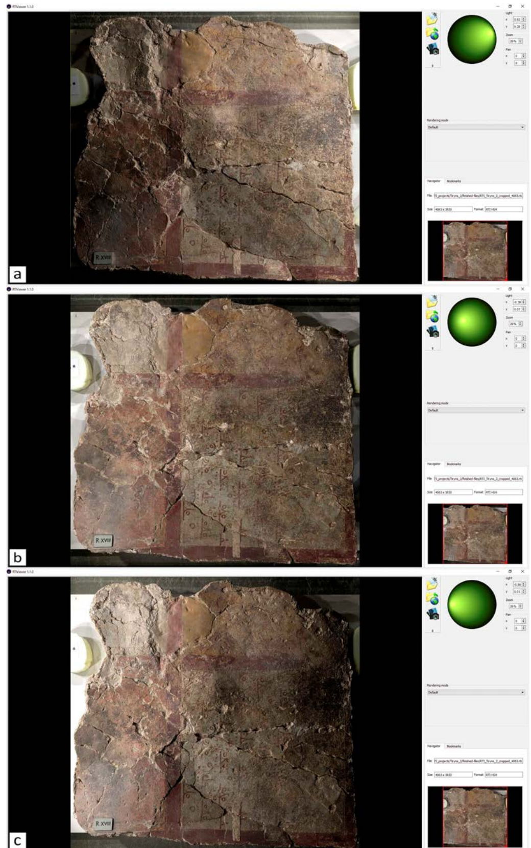
Figure 17. (a–c) Screenshots from RTViewer demonstrating the adjustment of the green sphere (top right) to simulate varying light directions for enhanced surface analysis.
