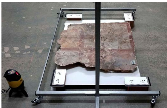
Figure 6. A line laser projecting a linear beam to facilitate the precise alignment of rulers on either side of the mural, ensuring the formation of a straight reference line.
